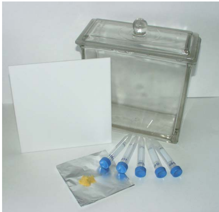
Fig.1: This still life shows 1. the chromatography tank (put 2 plates face-to-face) 2. the silica plate 3. the plastic tubes and a maize sample in powdered form
